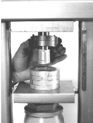
16) Photo of the result of the third draw. The cup should now be about 1 1/4" inside diameter and 1 5/8" tall.
