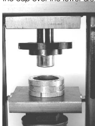
14) Photo of the result after the second draw. Unscrew punch and remove assembly, planish cup off punch.
