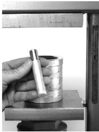
36) the result should be about 3" tall and 5/8" inside diameter.
