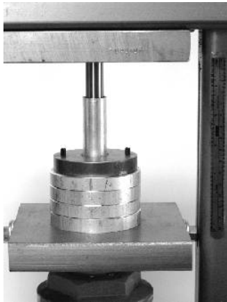
32) Draw, stopping when the lower platen reaches the 3 7/8" mark on the ruler.
